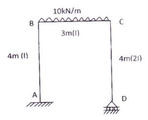
Q7) a) Generate the flexibility matrix [F] for coordinates 1, 2 and 3 of the cantilever beam shown in figure.[5]
